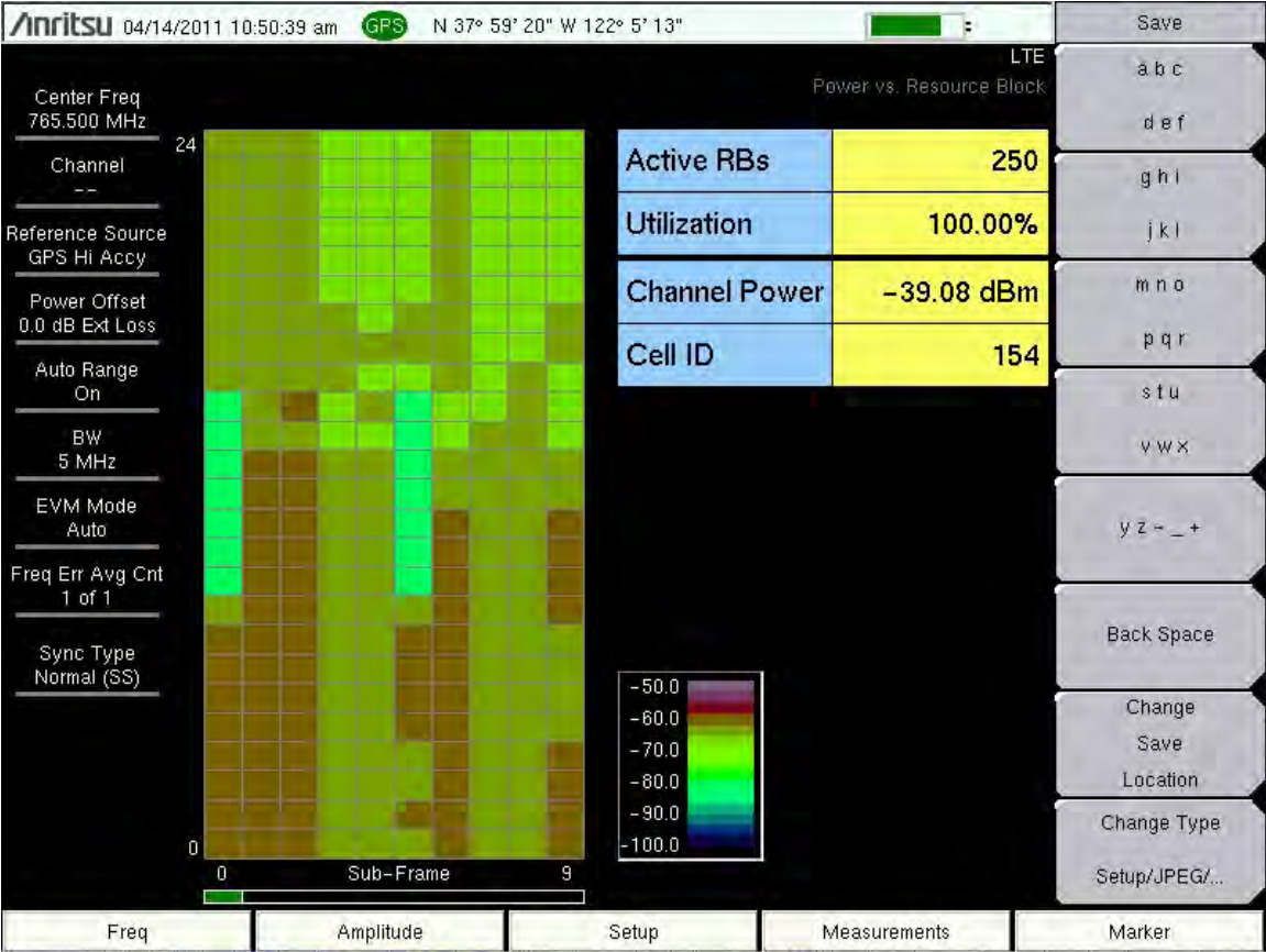
Anritsu Network Monitor showing very strong signal strength and 100% network utilization
