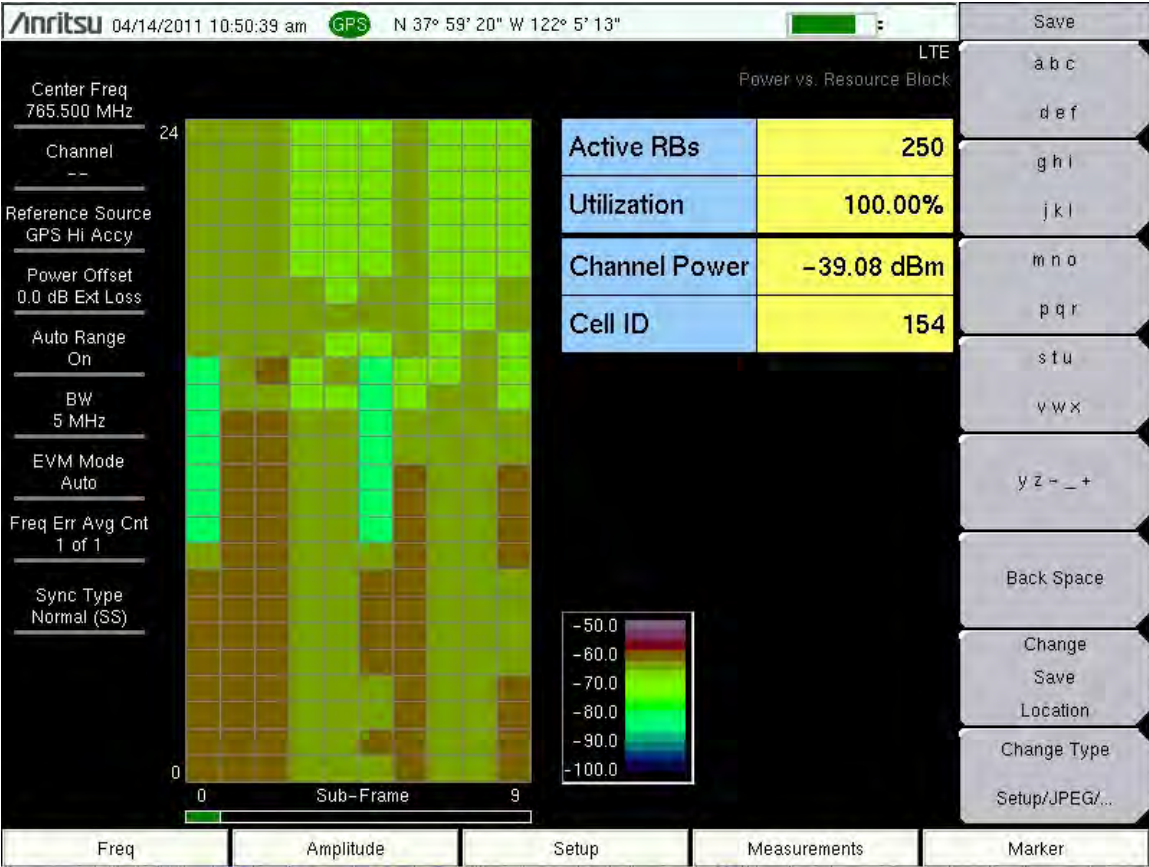
Diagram 1: Closest to the cell center, very strong signal, network is operating at 100% of its capacity
